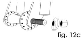
b. With a correctly sized socket, box, open-end or adjustable wrench, loosen the two axle nuts.
