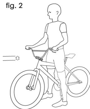
clearance of two inches (5 cm). A bike that you'll ride on unpaved surfaces should give you a minimum of four inches (7.5 cm) of standover height clearance. And a bike that you'll use for rough terrain, jumping or stunt riding should give you four inches (10 cm) or more of clearance.
