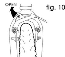
wheel is removed or reinstalled. When the brake quick release is in the released position, *the brakes are inoperative*. Ask your dealer whether you have a quick release on your brakes; and if you do, make sure that you understand the way the brake quick release works, and check *each time* to make sure both brakes work correctly before you get on the bike.
